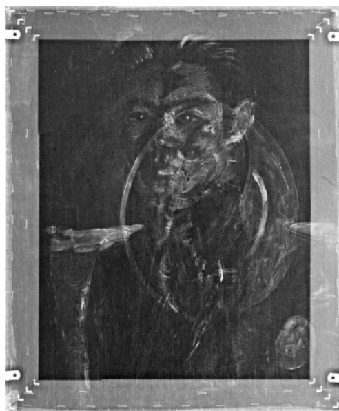
Fig. 15. The XRR image of Seafood rotated at 90° emphasises the brushwork and reveals rather a sketchy handling of paint in the area of the face. The lack of the X-ray absorption in the centre of the forehead suggests very little or no paint in that area
